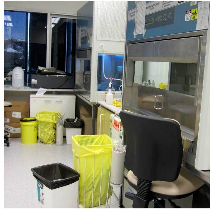
Cell culture laboratory illustrating two laminar flow cabinets for sterile cell culture..
